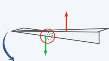
When you moved the paperclips to the front of the plane, the center of gravity moved in front of the center of lift. Now the weight pulls the front of the plane down. The airplane is still unstable!
