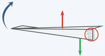
When you put paperclips on the back of the airplane, the center of gravity moved farther back. This extra weight pulls the back of the plane down, while the center of lift pulls the front up. The airplane is unstable!
