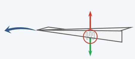
So where's the best place to put the weight? If the center of gravity is directly under the center of lift, then they balance each other. So for stable flight, the best place to put the weight is in the middle of the airplane!
