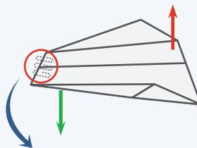
When you moved the paperclips to the front of the plane, the center of gravity moved in front of the center of lift. Now the weight pulls the front of the plane down. The airplane is still unstable!
