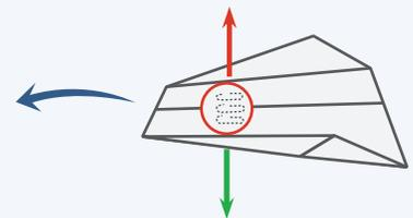
So where's the best place to put the weight? If the center of gravity is directly under the center of lift, then they balance each other. So for stable flight, the best place to put the weight is in the middle of the airplane!
